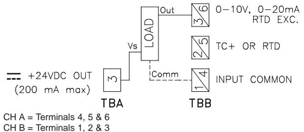
\* For two wire RTDs, install a copper sense lead of the same gauge and length as the RTD leads. Attach one end of the wire at the probe and the other end to input common terminal. Complete lead wire compensation is obtained. This is the preferred method. If a sense wire is not used, then use a jumper. A temperature offset error will exist. The error may be compensated by programming a temperature offset.
