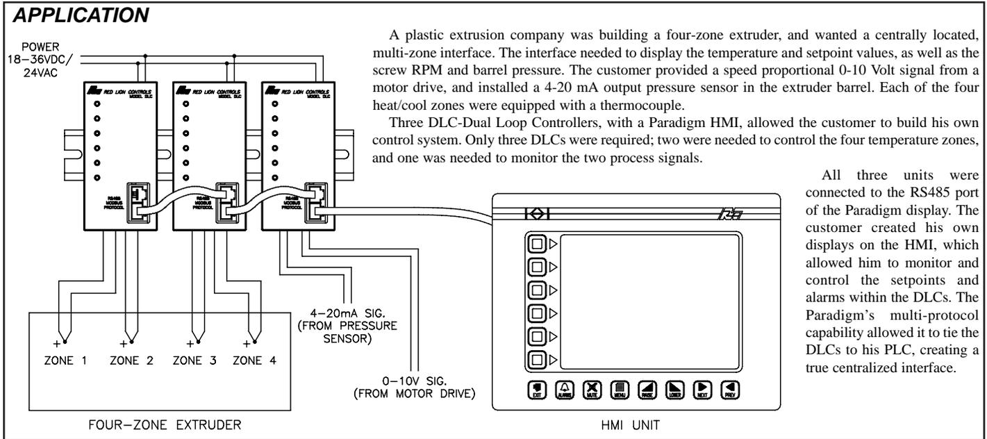
A plastic extrusion company was building a four-zone extruder, and wanted a centrally located, multi-zone interface. The interface needed to display the temperature and setpoint values, as well as the screw RPM and barrel pressure. The customer provided a speed proportional 0-10 Volt signal from a motor drive, and installed a 4-20 mA output pressure sensor in the extruder barrel. Each of the four heat/cool zones were equipped with a thermocouple.
