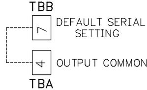
If using software selectable serial settings and the serial settings are unknown or forgotten, they can be temporarily reset to the defaults by connecting the "Default Serial Setting" terminal 7 to "Output Common" terminal 4 with a jumper.
