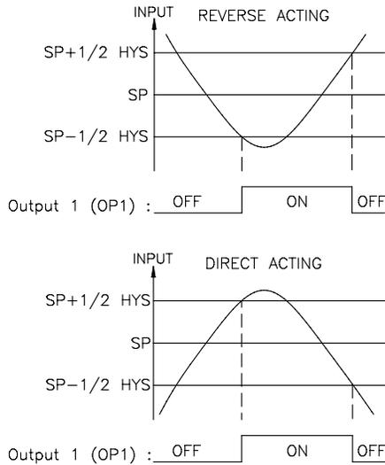
For heat and cool systems, OP1 Control Action is set to reverse (heat) and the Alarm 2 Action is set to cooling (OP2). The Proportional Band is set to 0.0 and the Relative Gain in Cooling to 0.0. The Deadband in Cooling sets the amount of operational deadband or overlap between the outputs. The setpoint and the On/Off Control Hysteresis applies to both OP1 and OP2 outputs. The hysteresis is balanced in relationship to the setpoint and deadband value.
