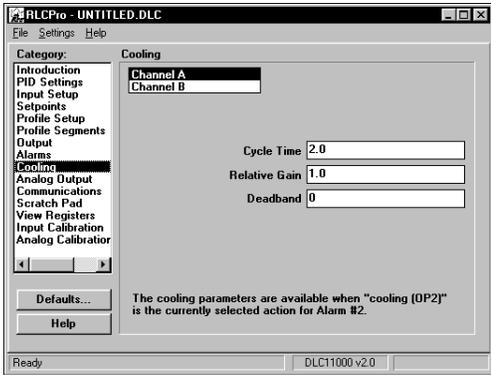
To enable Cooling in Heat/Cool applications, the Alarm 2 Action must first be set for Cooling. When set to cooling, the output no longer operates as an alarm but operates as an independent cooling output. The OP2 terminals are the same as AL2. Cooling output power ranges from -100% (full cooling) to 0% (no cooling, unless a heat/cool deadband overlap is used). The Power Limits in the Output category also limits the cooling power.
