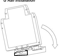
To install the IRMA on a "T" style rail, angle the module so that the top groove of the "foot" is located over the lip of the top rail. Push the module toward the rail until it snaps into place. To remove a module from the rail, insert a screwdriver into the slot on the bottom of the "foot", and pry upwards on the module until it releases from the rail.
