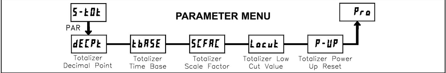
The totalizer accumulates (integrates) the Input Display value using one of two modes. The first is using a time base. This can be used to compute a time-temperature product. The second is through a user input or function key programmed for Batch (one time add on demand). This can be used to provide a readout of temperature integration, useful in curing and sterilization applications. If the Totalizer is not needed, its display can be locked-out and this module can be skipped during programming.
